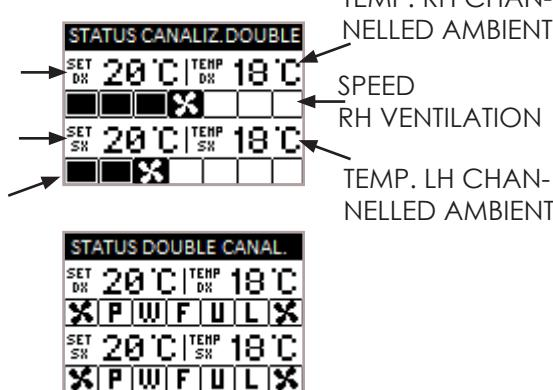
**i** When the POWERFUL function is enabled, in display status, you can also see that channelling is in this mode, as in the figure below.
